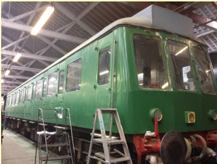
51382 inside the shed at Bury in primer during its repaint (Heritage Painting)
